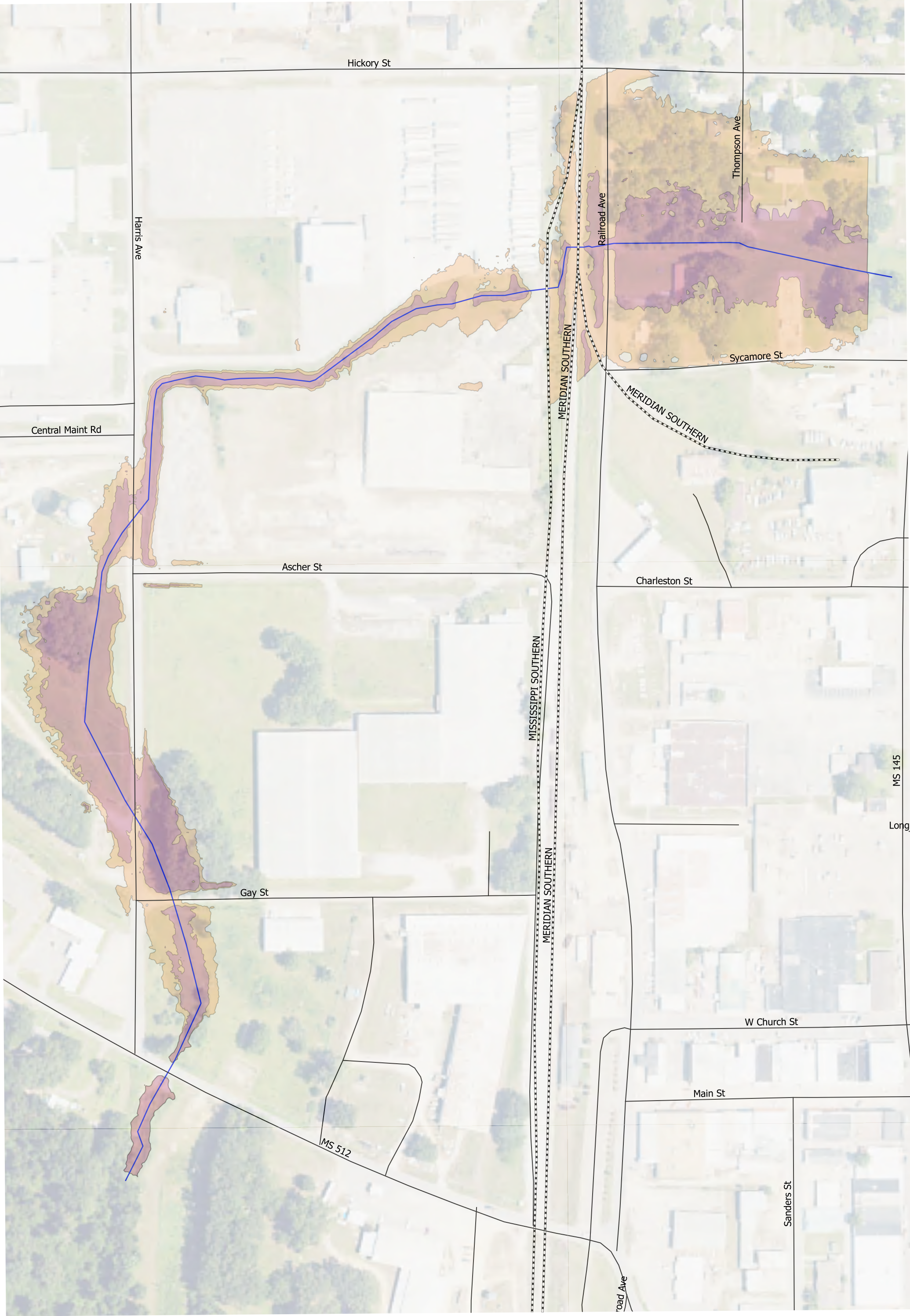
Harris/Dart Channel Inundation Boundary for 25-yr Flow Orange = Existing, Red = Proposed
