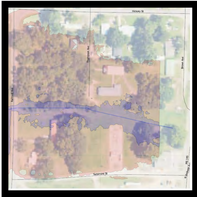
Figure 9 -Inundation area of the 25-year flow for existing conditions (in red) and proposed conditions (in blue).
